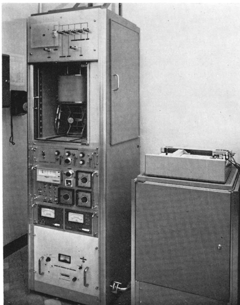
Fig. 4. General view of the apparatus. Left cabinet, from top to bottom: gas manifold, liquid thermostat surrounding the vertical tubes of the balance (behind the transparent door closing the air bath), balance electronics, temperature controllers, timers, vacuum gauges, Texas gauge. Right cabinet: inside, rotating pump and thermostat-cryostat; on the top, X-Y recorder.
